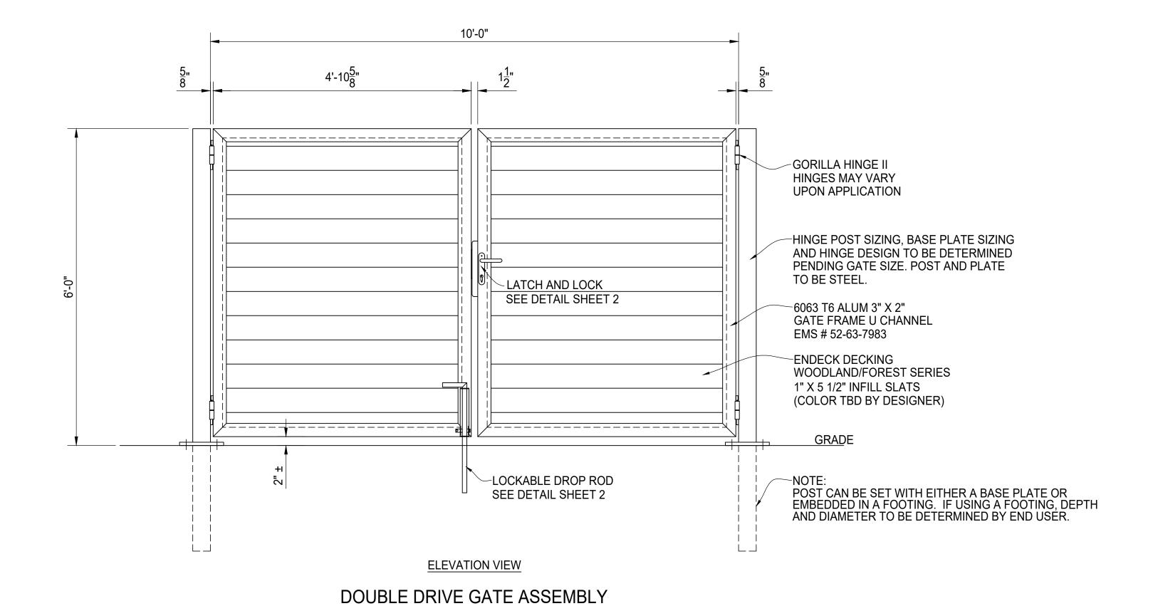
SEE DETAIL SHEET 2 FOR HINGE, LATCH AND DROP ROD
